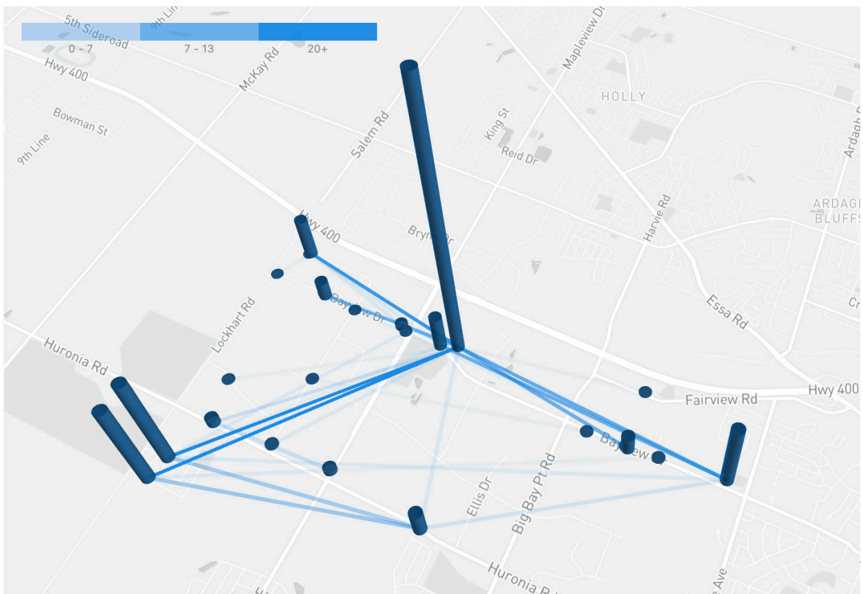
FIGURE 9: ORIGIN-DESTINATION PAIRS OF ON-DEMAND TRIPS, WHICH COULD REVEAL OPPORTUNITIES TO INTRODUCE FIXED ROUTE SERVICE.
